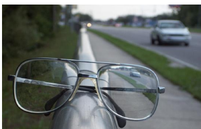
Figure 25.6.12: A car viewed through a concave or diverging lens looks upright. This is a case 3 image. (credit: Daniel Oines, Flickr)
