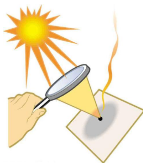
Figure 25.6.2: Sunlight focused by a converging magnifying glass can burn paper. Light rays from the sun are nearly parallel and cross at the focal point of the lens. The more powerful the lens, the closer to the lens the rays will cross.
