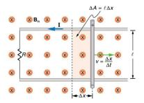
We have seen one case of motional EMF early on in this unit when discussing the Hall Effect. Consider a conductor moving through a magnetic field as shown in the figure above. As the conductor is moving through the field, EMF is induced according to Faraday's law:
