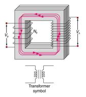
For a simple transformer such as the one shown above, the output voltage depends almost entirely on the input voltage and the ratio of the number of loops in the primary and secondary coils. Faraday's law of induction for the secondary coil gives its induced output voltage to be:
